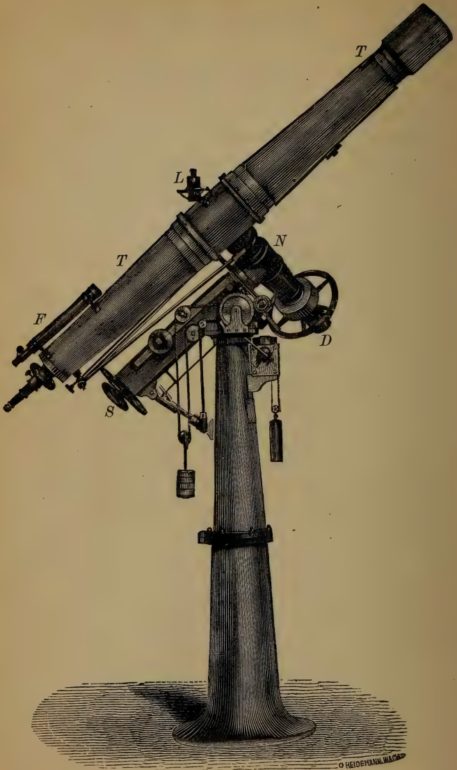
FIG. 37.—EQUATORIAL TELESCOPE POINTED TOWARD THE POLE.
